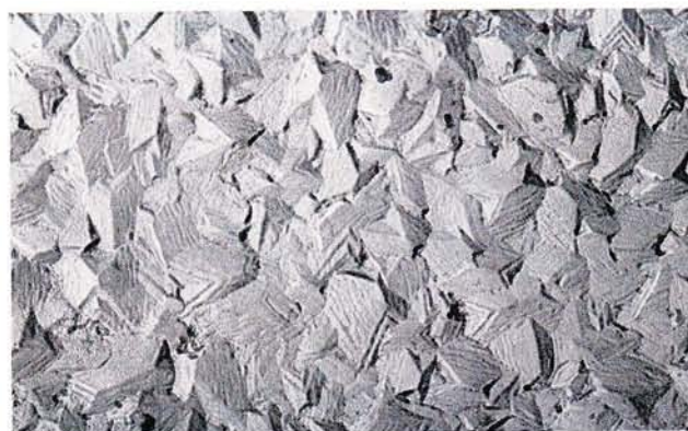
Electron photo-micrograph of replica showing the crystalline structure of conducting tin oxide at 50,000 times magnification.
